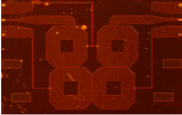
Fig. 10. Photograph of the second fabricated filter.
