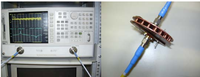
Fig. 20. Network Analyzer HP 8720ES with excitation and measure probes.
